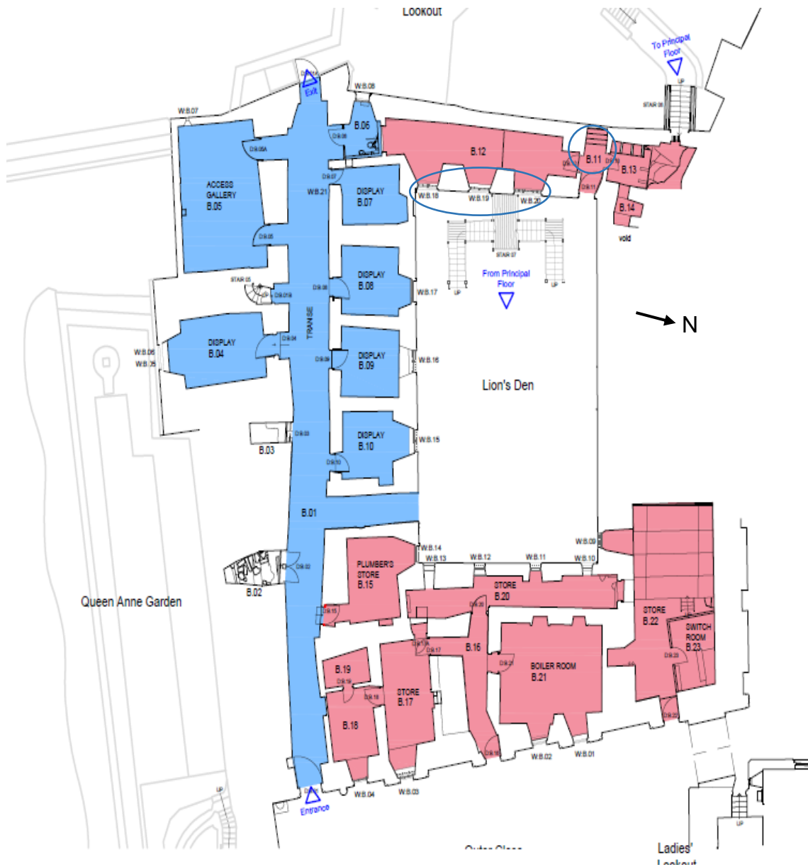
Fig 1. Plan of the vault level of the buildings surrounding the Lion's Den. The timber lintols are within B.11, at the west end of the room, and above windows W:B.18, W:B.19 and W:B.20 in B.12.
