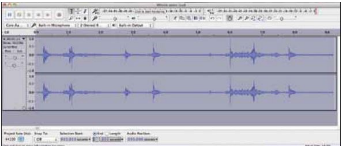
Figure 10: Sound profile of Type 3 sling bullet in flight, the peaks denote the buzz sound as the bullet tumbles through the air.
