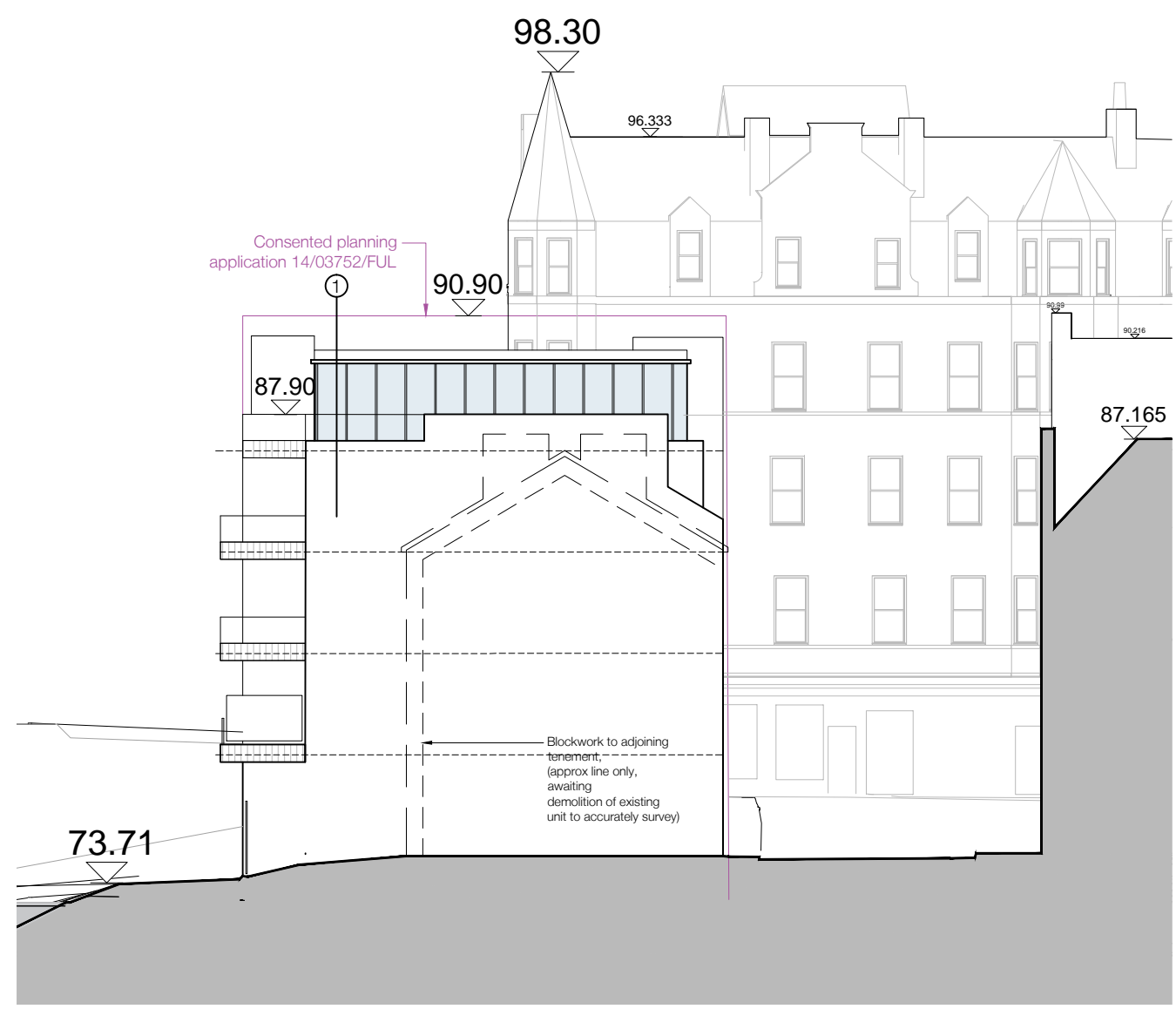
Home Terrace West Side Elevation - 1:200 @ A3
