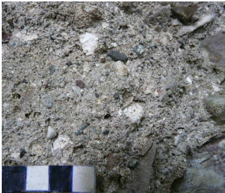
Figure 8 (above) – Kinclaven Castle; core mortar of south-east wall clearly displaying large angular and white probable limestone kiln-relict clasts, and rounded lithic temper inclusions. Scale 10mm; photograph M. Thacker.
