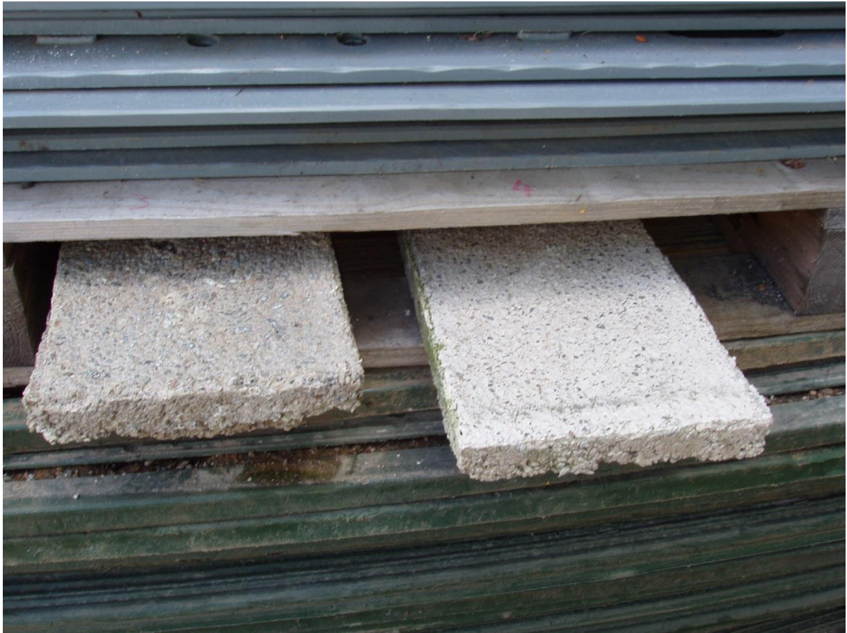
Left hand sample is the preferred wash grit mix (3:3:1 Bluehill 6mm Chip, Rothes Glen sand, St. Astier NHL5 Lime)
