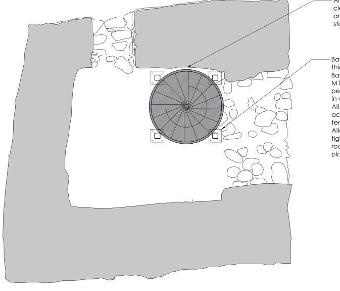
All loose stone and debris to be cleared away from base of stair and scrapped back to sound stone below base plates.
